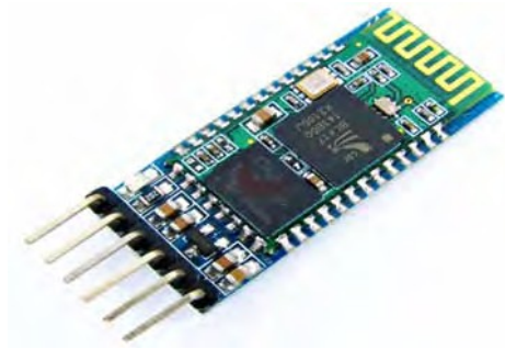
Figure 2.4 Physical Form of Bluetooth Module HC-05 (Source: Ratna Dewi, Ramiati; 2011: 48)
