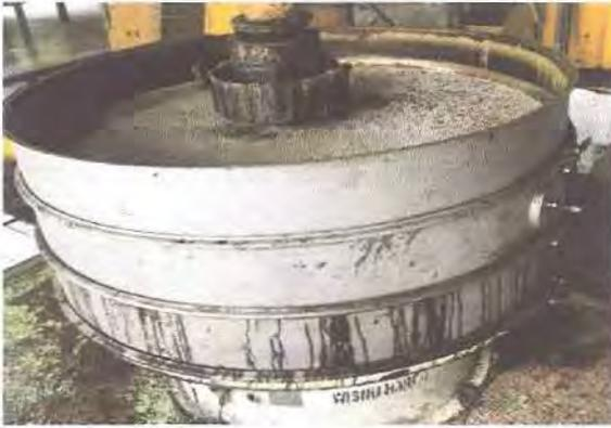
**Gambar 3.14. *Vibrating Sweco***
