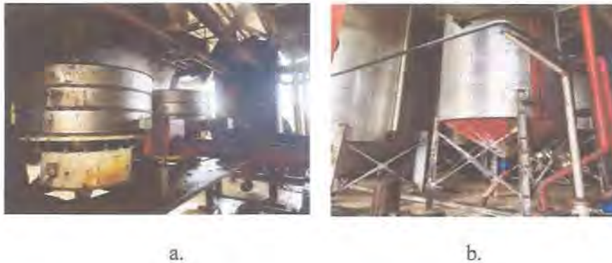
Gambar 3.11. (a) Oil Vibrating Screen (b) Crude Oil Tank
