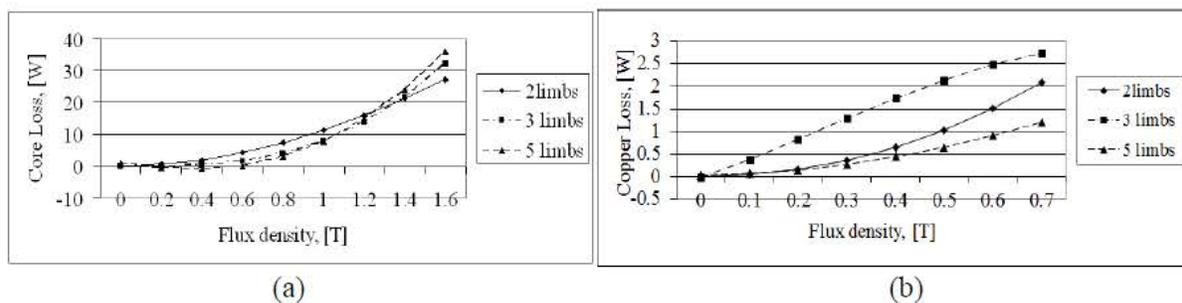
Figure 5 (a) Core loss and (b) Copper loss of transformer under different limb
