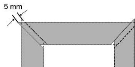
Figure 3 Transformer core type with stagger yoke
