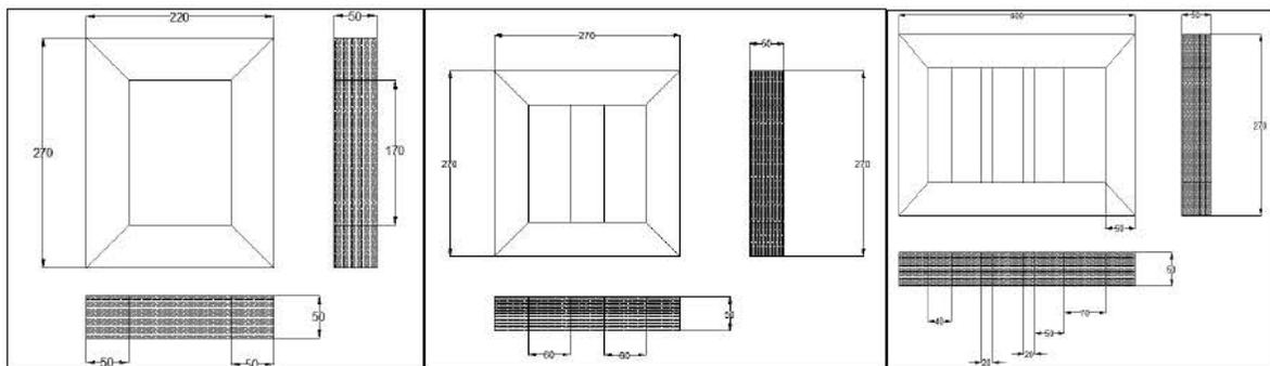
Figure 2 Dimension of two, three and five limbs transformer core design (mm)
