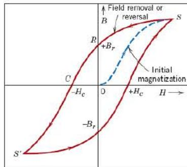
Figure 1 The B vs. H behavior for ferromagnetic material [6]
