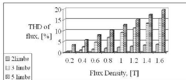
Figure 6 Total harmonic distortion of transformer under different limb
