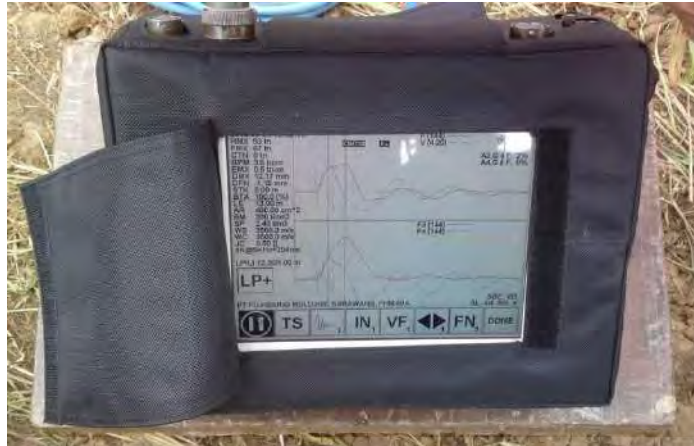
Gambar 2.1 Pile Driving Analyzer (ASTM D-4945-1996)
