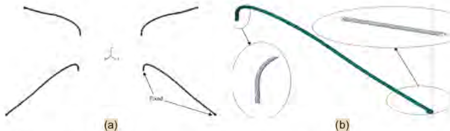
Figure 3. (a) Boundary condition of wires in ABAQUS, (b) Meshed wire for ABAQUS analysis
