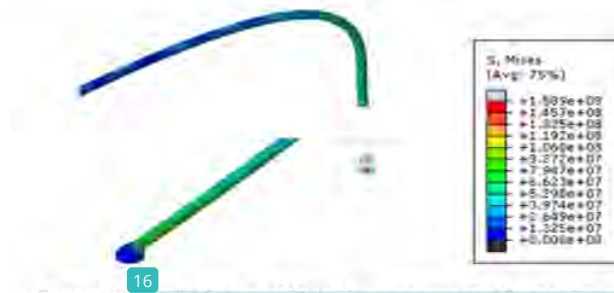
Figure 9. Detailed view of Von-Mises stress distribution for wire 1
