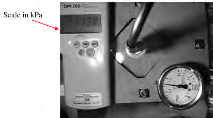
1 Figure 4.16 Pressure Validation on top centre position of pressure sensor at full filled.
