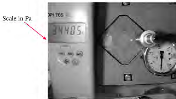
1 Figure 4.15 Pressure Validation on top corner position of pressure sensor at full filled.
