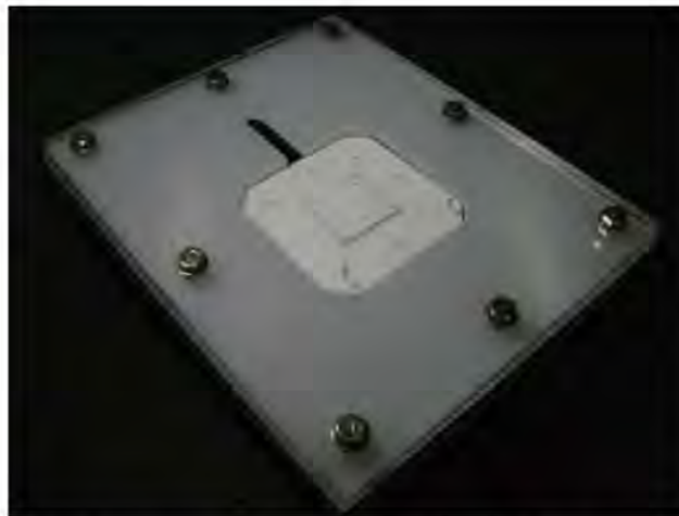
Figure 3.16 Detailed construction of mould of scale-up eight-wire PBGA model with centre inlet.
