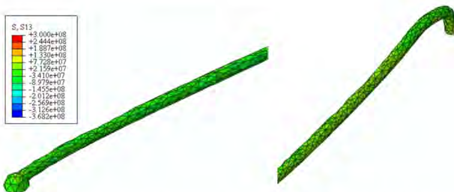
Figure 4.78 Detailed view of maximum Shear stress (S13) distribution for Wire 4 of simulation optimization result.
