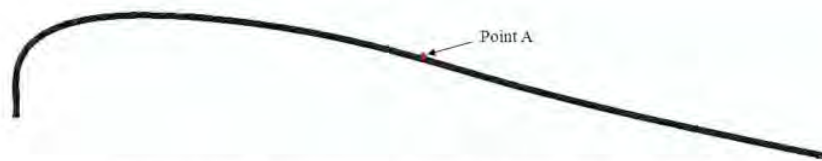
Figure 4.23 Measurement of wire deformation at Point A.
