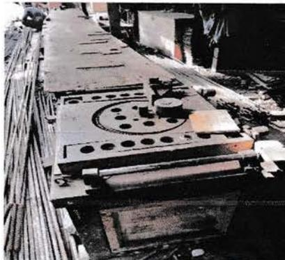
Gambar 3.5 Bar Bending
