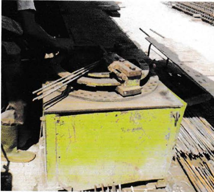
**Gambar 13. Bar Bending**
