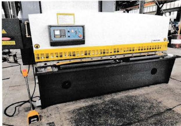
Gambar 3.3. Mesin *Metal Shearing*
