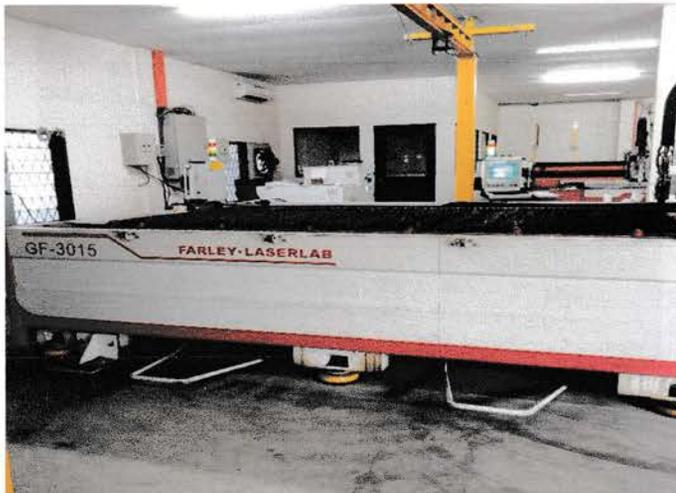
Gambar 3.2. Mesin *Fiber Laser Cutting*
