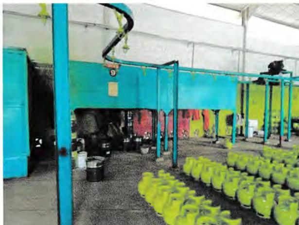
**Gambar 3.17 Gantungan *Trolley* Pada *Chain Conveyor***
