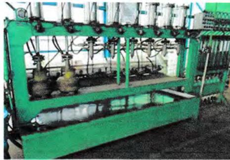
**Gambar 3.35 Visual Mesin *Hydrostatic Test***
