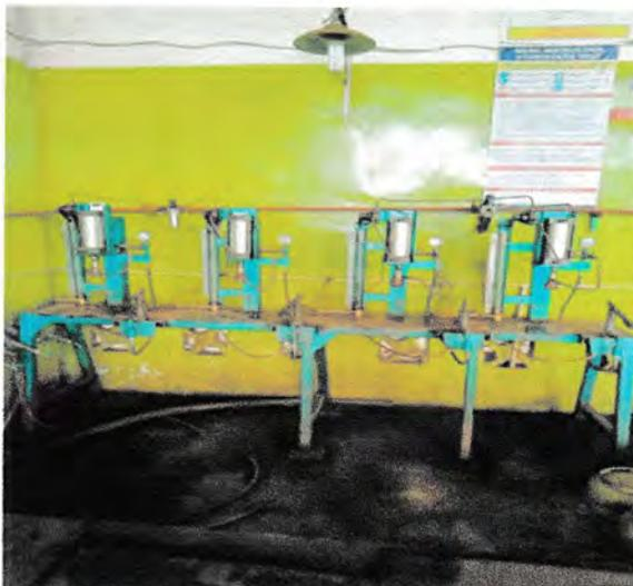
**Gambar 3.12 Hydrostatic Test**
