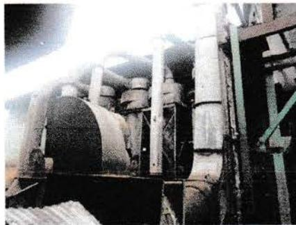
**Gambar 3.42** LTDS (*Light Tenera Dust Seperator*)
