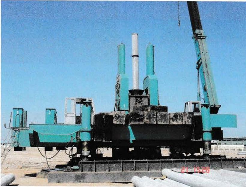
Gambar 2.2 Hydraulic Static Pile Driver (DTZ Series)
