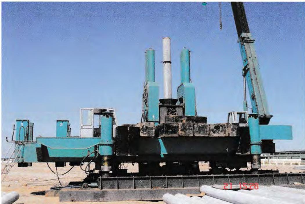
Gambar 2.2 Hydraulic Static Pile Driver (DTZ Series)
