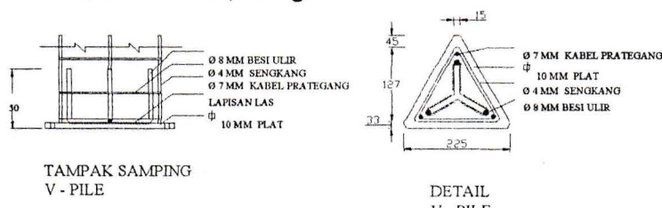
gambar 8. Penampang V-Pile
