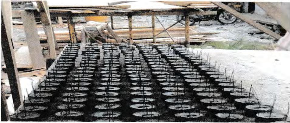
**Gambar 3.5 Beton Decking**
