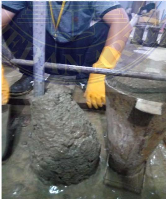
Gambar 2.5 Slump test
