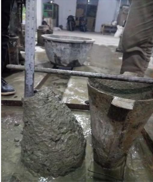
Uji slump beton
